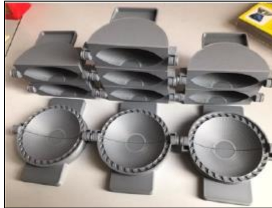
Figure 3. Printed curry puff mould using 3D printer
