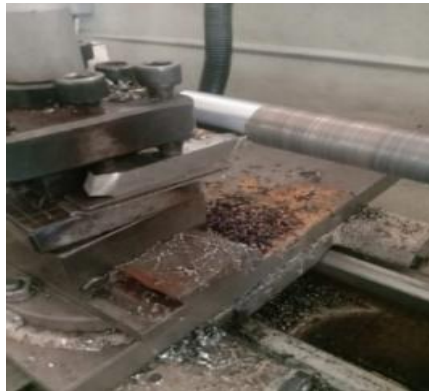
Figure 14. Fabrication of the shaft end for the cylinder wall section
