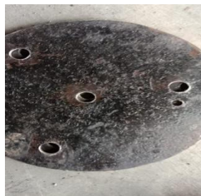
Figure 10. Fabrication of the iron plate separator circle
