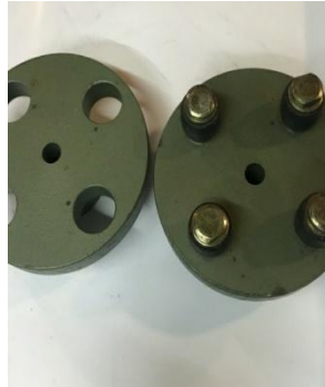
Figure 20. Fabrication of the fixed coupling hole
