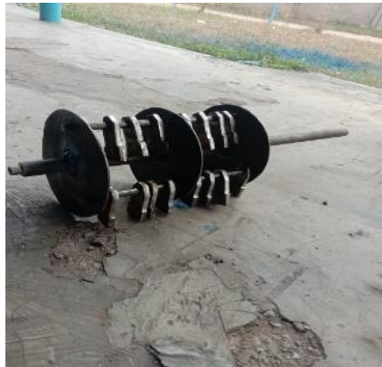
Figure 17. Fabrication of the hammer reinforcing steel lock
