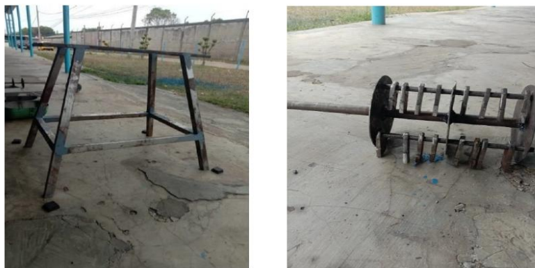
Figure 2. Frame and hammers of the glass waste crusher hammer mill machine.
