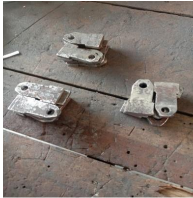
Figure 9. Hammer hole fabrication
