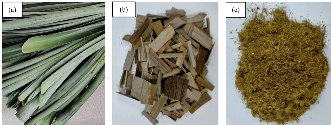
Figure 3. Pineapple leaves: (a) Fresh leaves, (b) Chopped leaves before grinding, and (c) Ground pineapple leaf powder.
