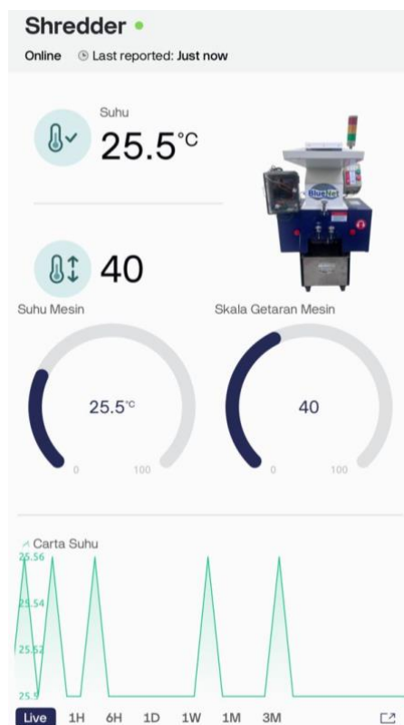
Figure 4. Blynk mobile application interface showing real-time monitoring of shredder motor temperature, vibration scale, and status visualization.
