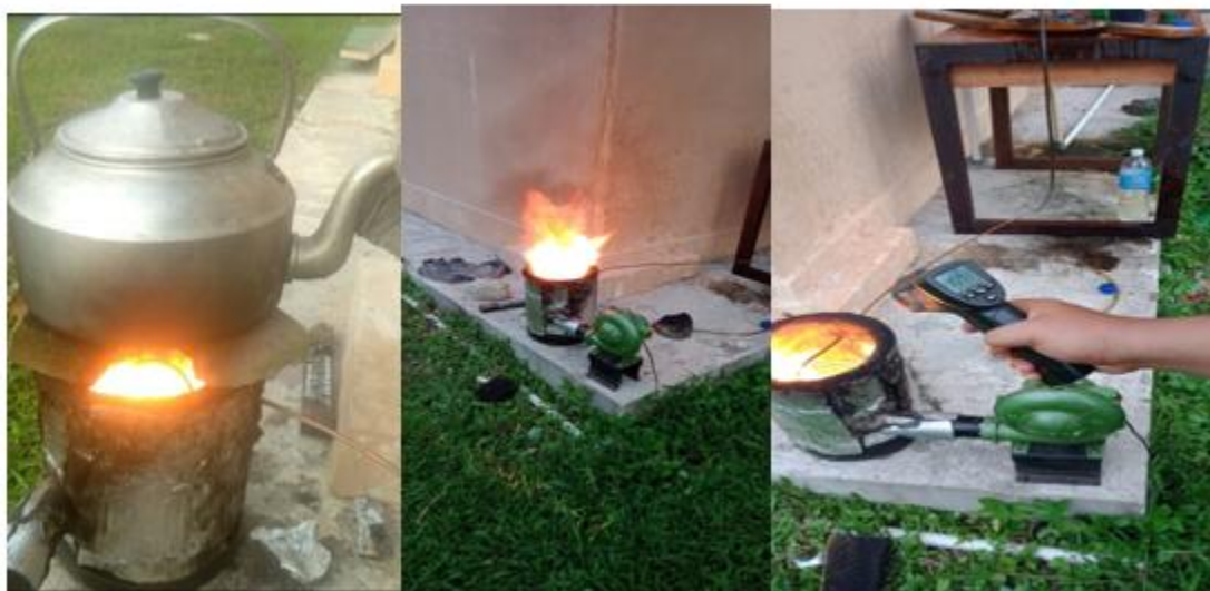
Figure 1. The performance testing of the burner focused on three main parameters: flame temperature, heating rate, and combustion rate. These parameters were measured to evaluate the influence of different fuel variations (waste oil and its mixtures with gasoline) on burner efficiency.
